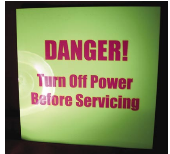
The same warning sign illuminated with a 60-watt blacklight bulb in a darkened room.
