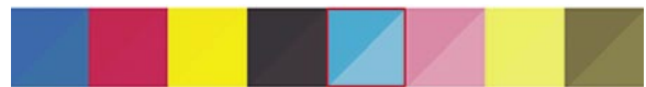
EXPOSED SAMPLE: This chart displays before and after color measurements. The left half of each square shows the color before UV exposure. The right half portrays the color after exposure. No visual changes in the 100% CMYK squares are apparent. The 50% CMYK squares exhibit a small amount of Cyan and Magenta fade. Overall performance was excellent.
